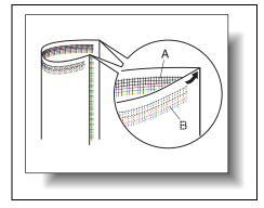
8 If horizontal lines A and B are angled as shown at the right, touch to specify the desired negative adjustment for  $\theta$ (between -1 dot and -10 dots).
